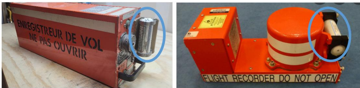
Figure 1: HF-ULB Installations on various recorders
